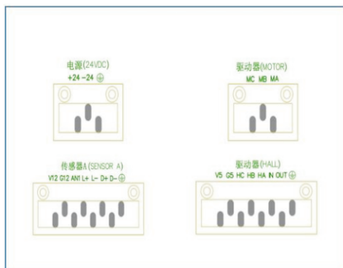
SMK-30-4P SMK-60-4P SMK-80-4P 单探头接线示意
